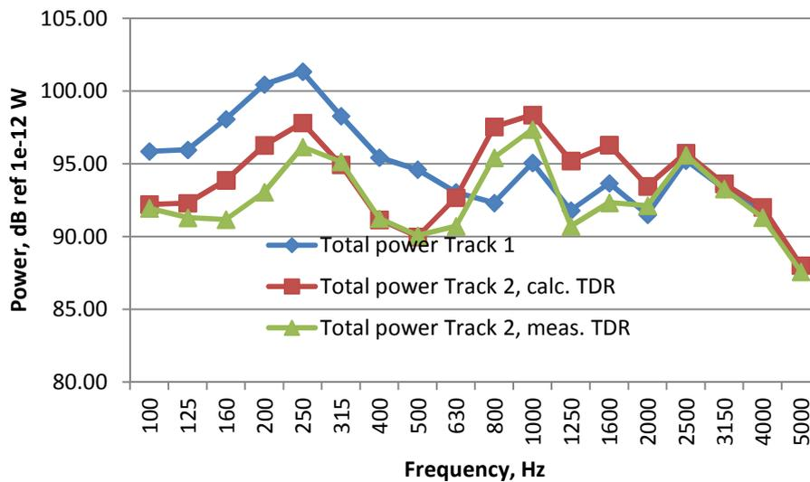
**Figure 7-8 : Total sound power for Tracks 1 and 2 (ISVR calculations)**
