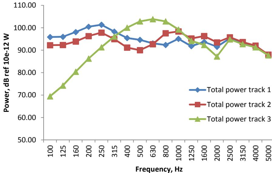
**Figure 4-3 : Total radiated power (track + wheel) for different tracks, calculated decay rates (ISVR calculations at 160 km/h using TSI roughness as total roughness))**
