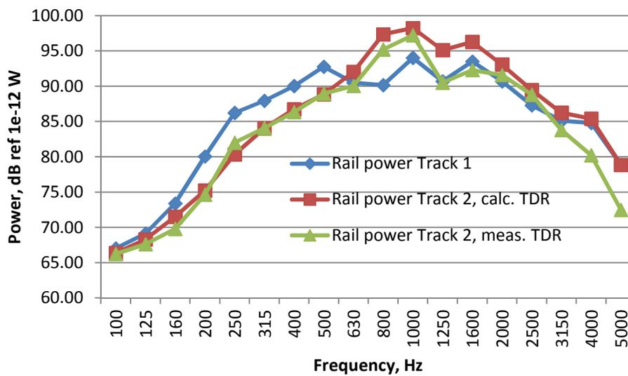
**Figure 7-6 : Rail sound power for Tracks 1 and 2 (ISVR calculations)**
