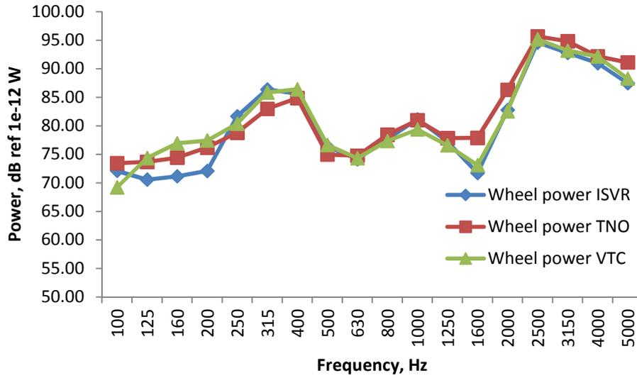
Figure 7-4: Wheel sound power case 2 (VB2N on track 2 at 160 km/h)
