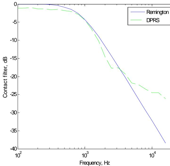
**Figure 2-1 : Contact filtering effect for  $a=5.69$  mm and  $v=100$  km/h**
