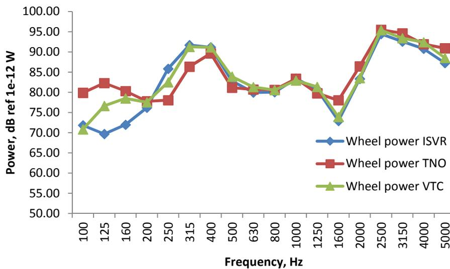
**Figure 7-3 : Wheel sound power case 1 (VB2N on track 1 at 160 km/h)**
