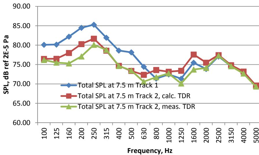
**Figure 7-9 : Total sound pressure for Tracks 1 and 2 (ISVR calculations)**
