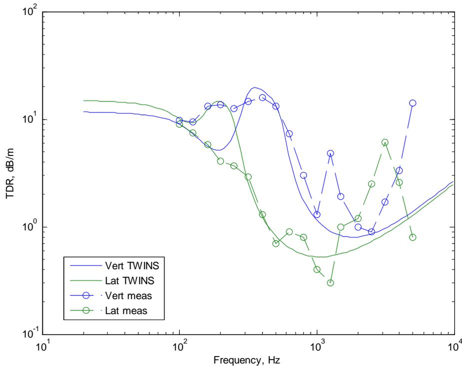
Figure 7-5: Comparison of measured and calculated decay rates, bi-bloc track, ISVR
