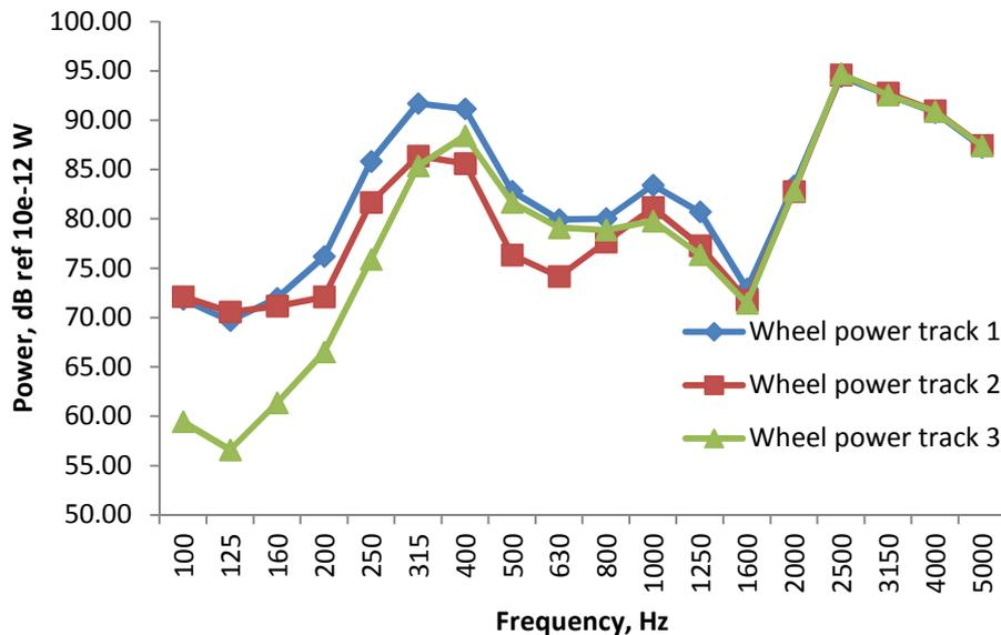
**Figure 4-2 : Wheel (VB2N) radiated power for different tracks (ISVR results at 160 km/h using TSI roughness as total roughness)**
