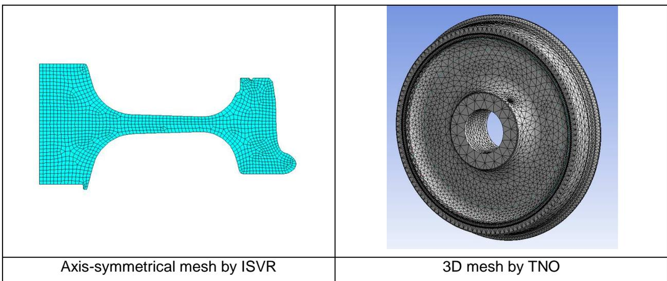
**Figure 7-2: Meshing of VB2N wheel performed by ISVR and TNO**
