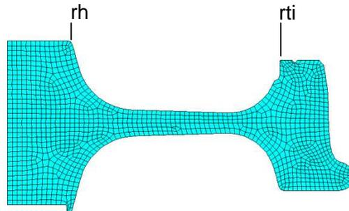
**Figure 3-1 : Wheel mesh example (VB2N wheel), indication of hub radius (rh) and inner tyre radius (rti), meshing performed by ISVR**
