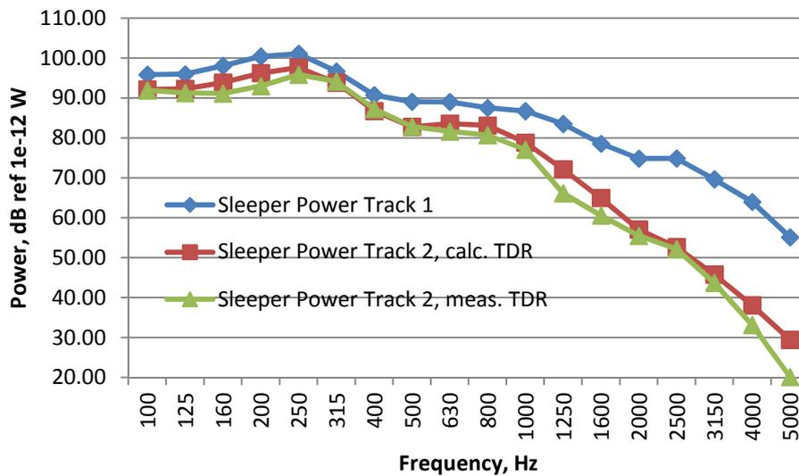
**Figure 7-7 : Sleeper sound power for Tracks 1 and 2 (ISVR calculations)**
