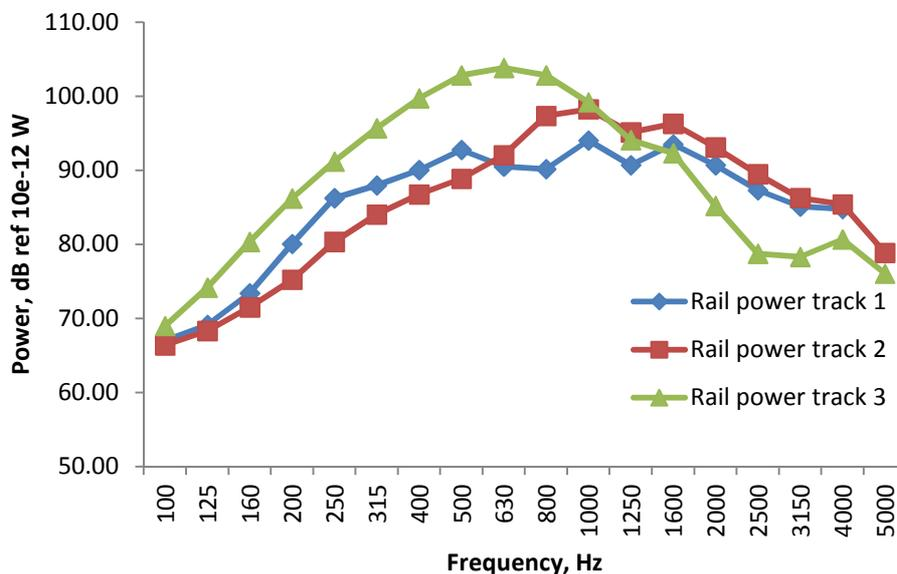
**Figure 4-1 : Rail radiated power for different tracks, calculated decay rates (ISVR calculations at 160 km/h using TSI roughness as total roughness), see section 4.1 for details on the various tracks.**
