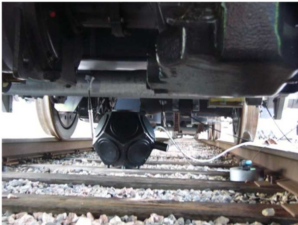
Artificial source in bogie cavity
