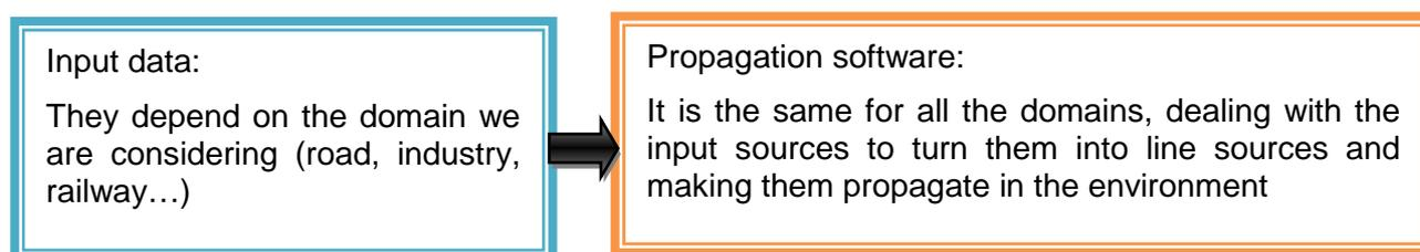
**Figure 2-1: The two main steps in the CNOSSOS methodology**
