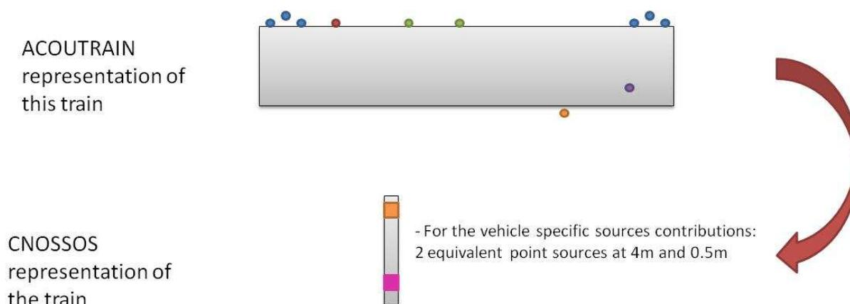
**Figure 3-3: Noise source representation in ACOUTRAIN (distributed on the virtual vehicle) and in CNOSSOS**
