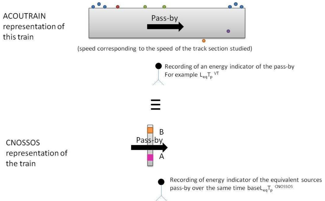
**Figure 3-4: Principle of definition of CNOSSOS inputs from ACOUTRAIN simulation**
