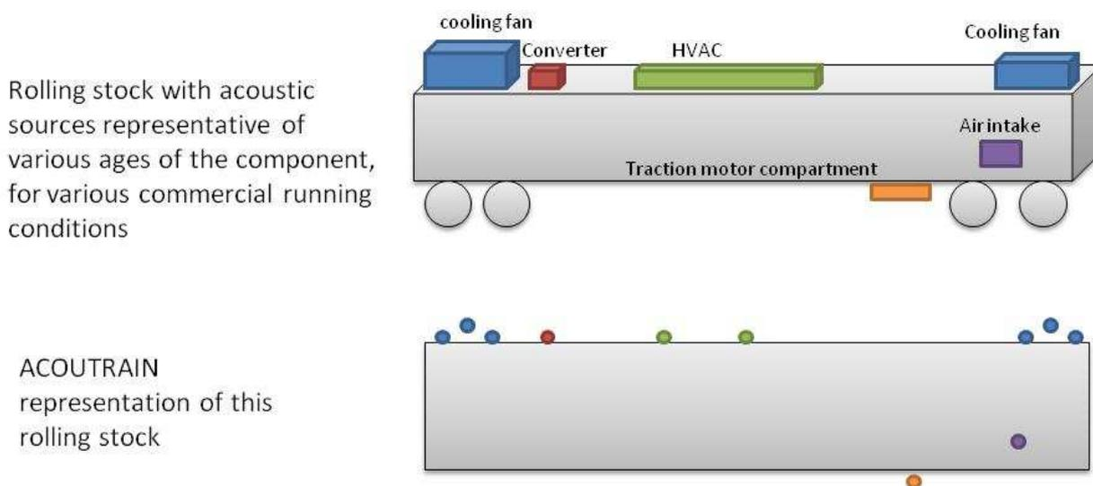
**Figure 3-2: Rolling stock definition in ACOUTRAIN for CNOSSOS purposes**
