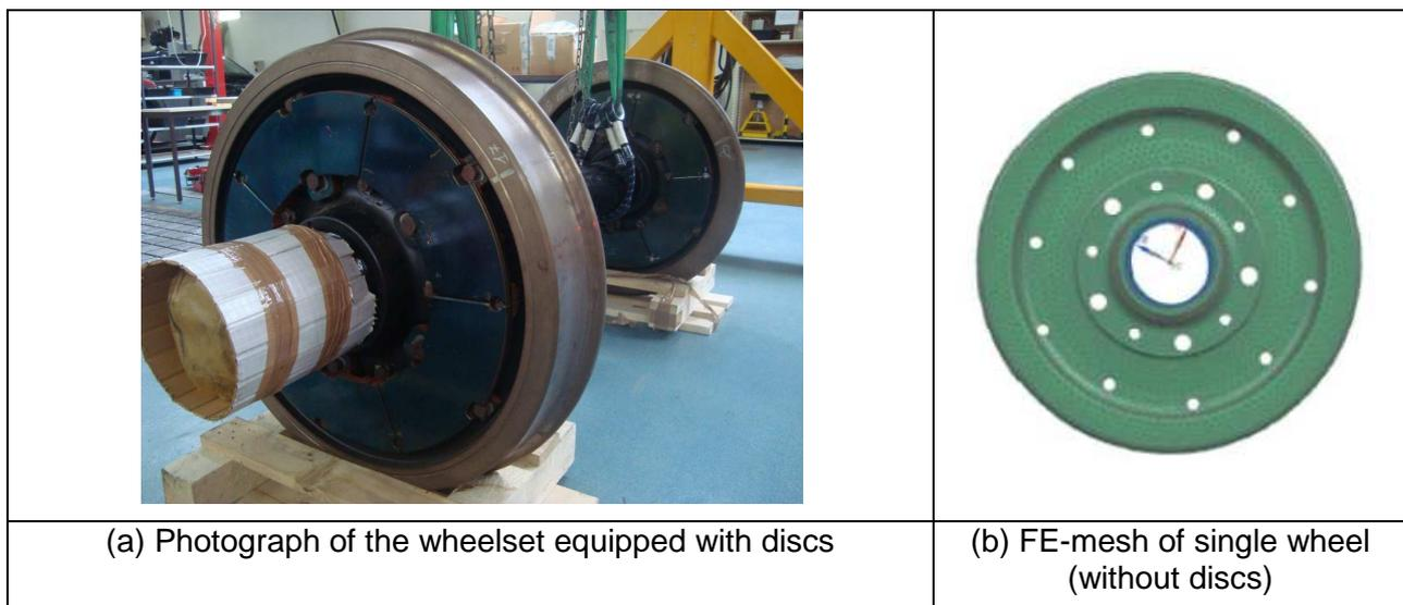
**Figure 3-1: ETR wheelset supplied by ALSTOM for Acoutrain**
