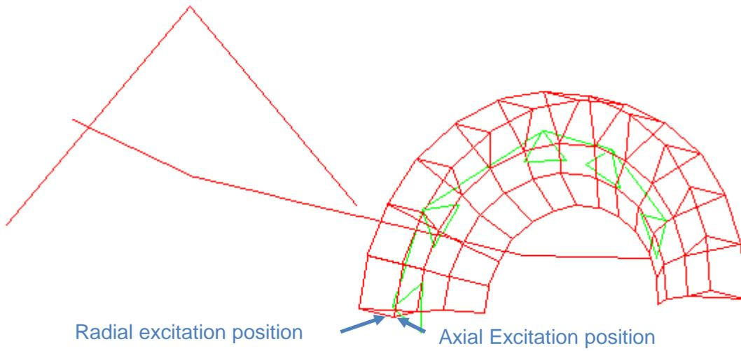
**Figure 3-4: EMA mesh example**
