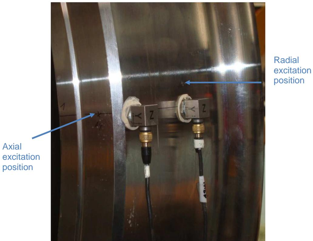
**Figure 3-5: Position of accelerometers**
