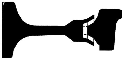
**Figure 3-2: Sketch of a resilient wheel section**
